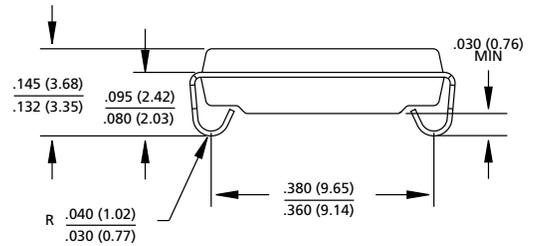
**NOTE:** 1. All dimensions in inches (millimeters) **MAX** or typical where noted.
