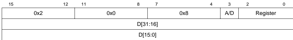
Figure 5-19. WAREG/WDREG Command Format
