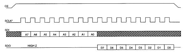
The address byte is always the first byte entered after CE is driven high. The most significant bit (A7) of this byte determines if a read or write will take place. If A7 is "0", one or more read cycles will occur. If A7 is "1", one or more write cycles will occur.
