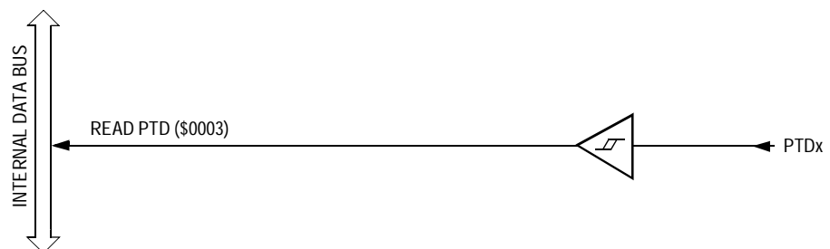
Figure 15-12. Port D Input Circuit
