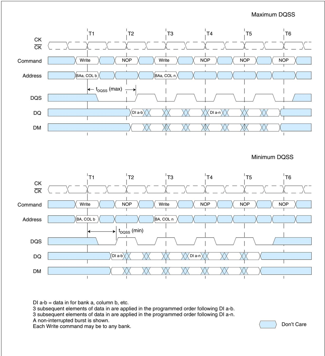
Figure 19 Write to Write (Burst Length = 4)
