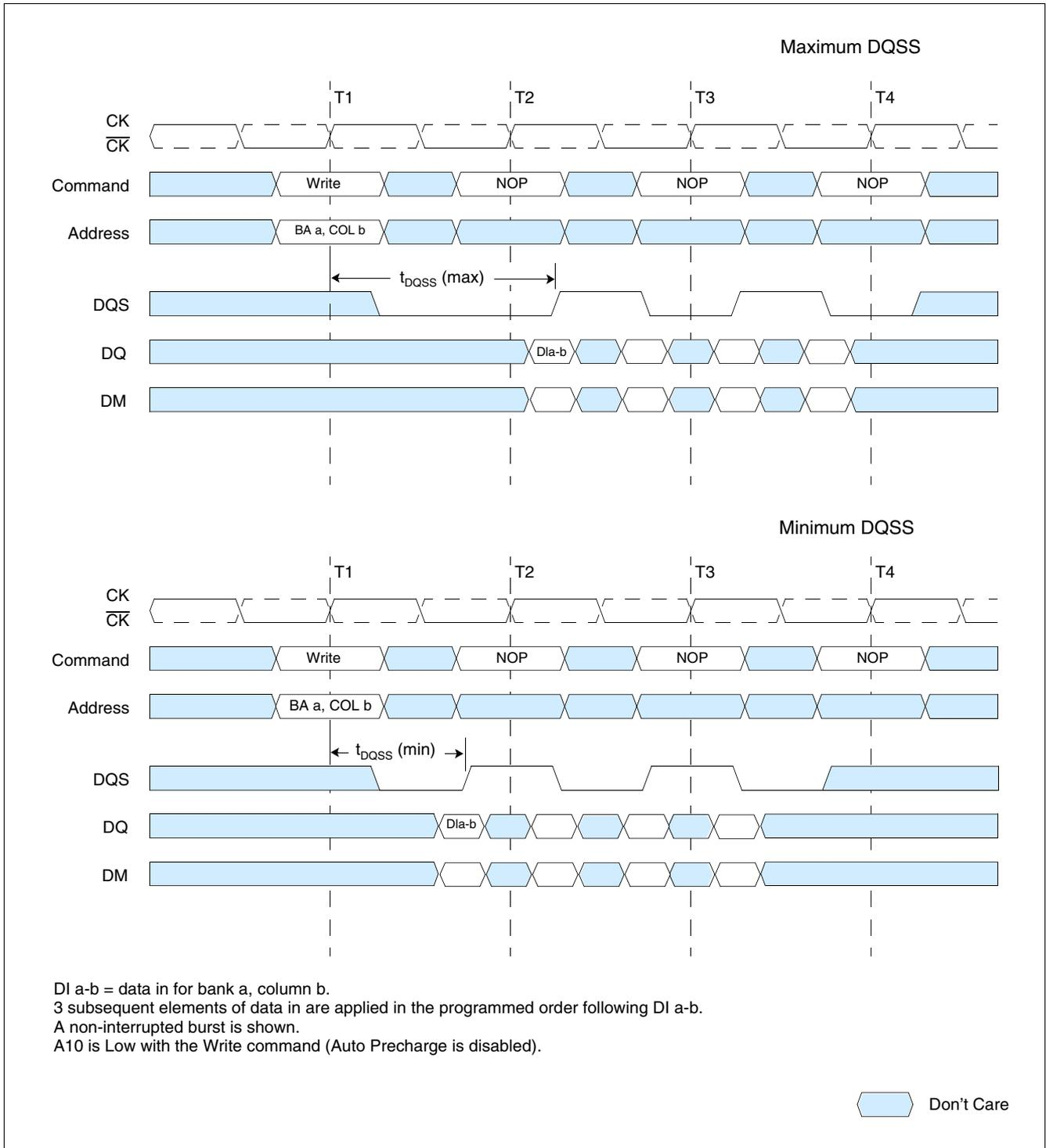
Figure 18 Write Burst (Burst Length = 4)
