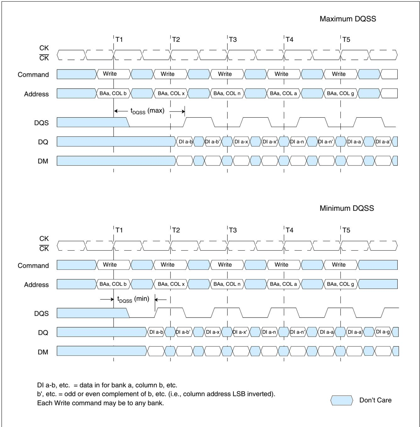
Figure 21 Random Write Cycles (Burst Length = 2, 4 or 8)
