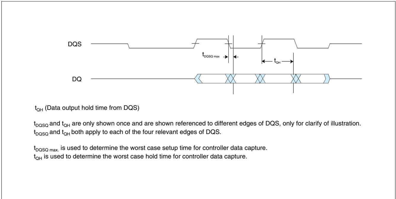
Figure 39 Data Output (Read), Timing Burst Length = 4
