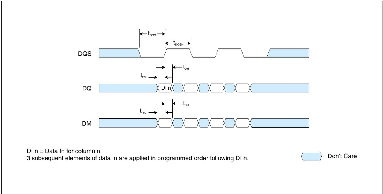
Figure 38 Data Input (Write), Timing Burst Length = 4
