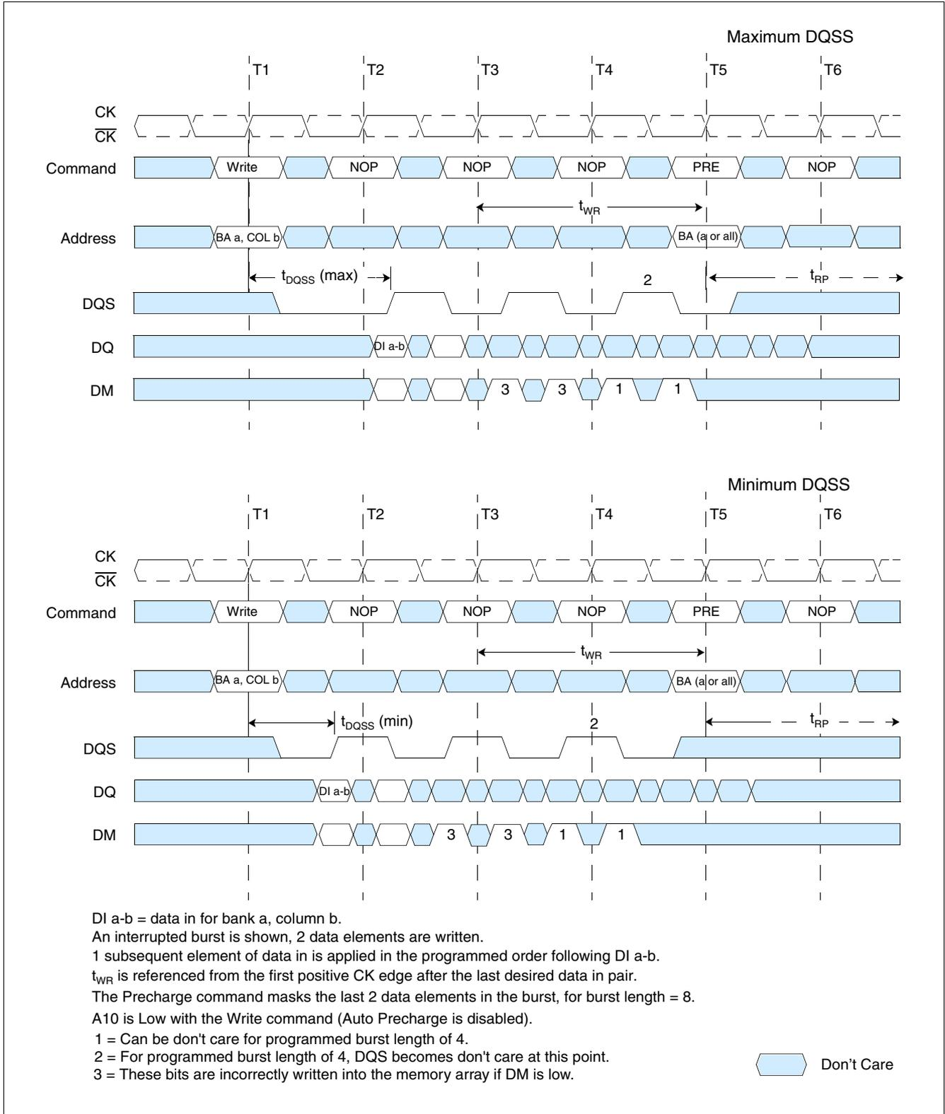
Figure 27 Write to Precharge: Interrupting (Burst Length = 4 or 8)
