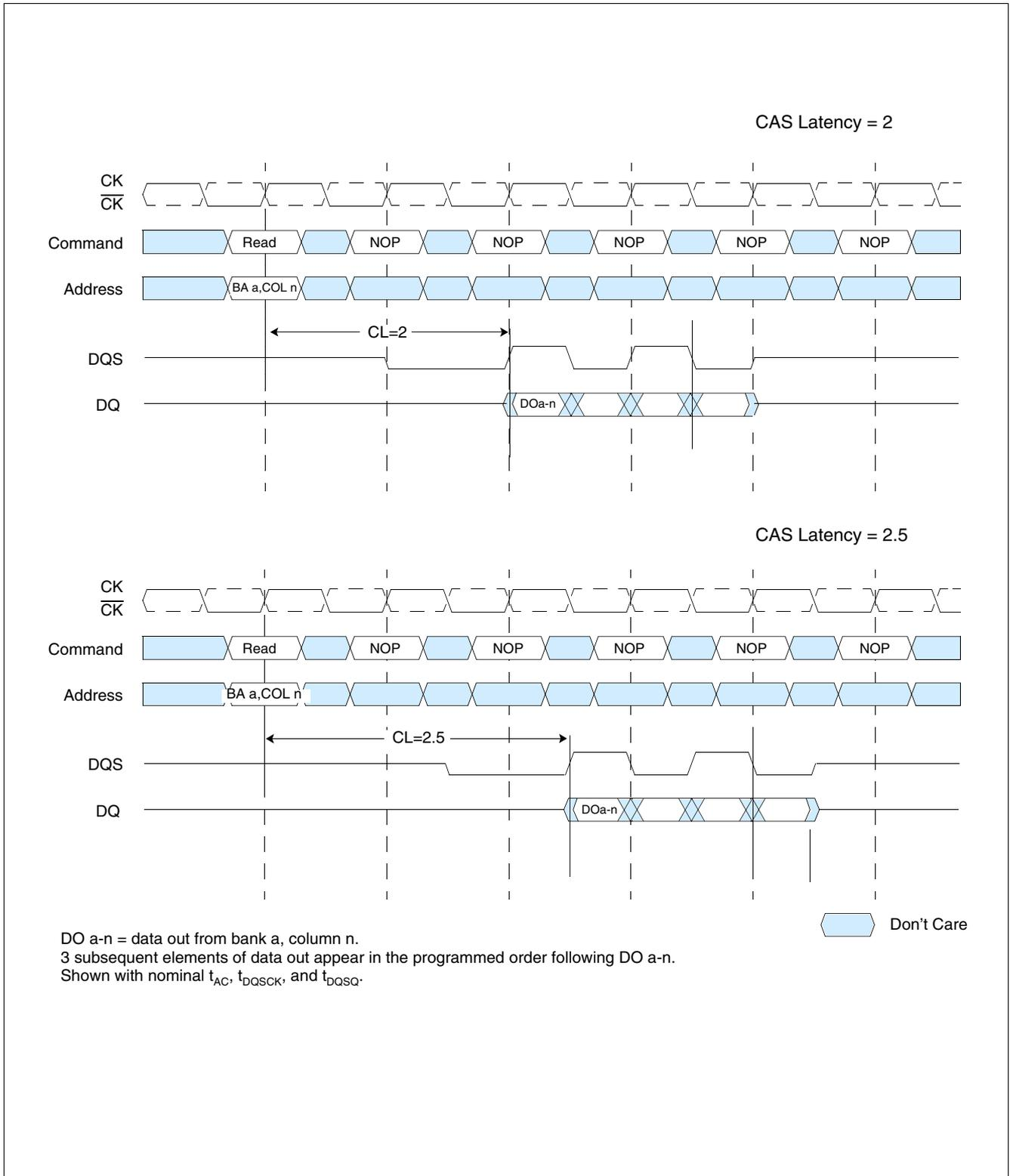
Figure 10 Read Burst: CAS Latencies (Burst Length = 4)
