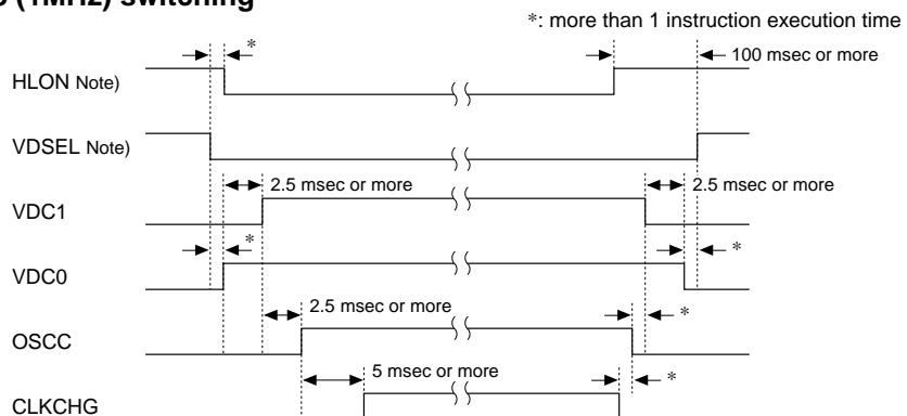
Note) When the reduce mode is used. However, when using the reduce mode in the LCD system voltage circuit ( $VCSEL = "1"$ ), HLON should be set to "1".
