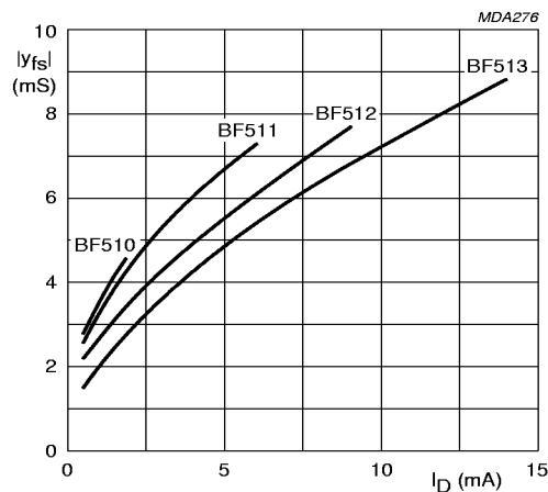
Fig.3  $V_{DS} = 10 \text{ V}$ ;  $f = 1 \text{ kHz}$ ;  $T_{amb} = 25^\circ\text{C}$ ; typical values.
