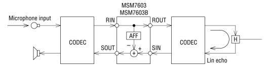
Example 3: Canceling of both acoustic and line echo (to handle both acoustic echo from line input and line echo from microphone input)
