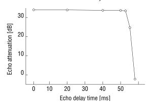
Measurement Conditions : RIN input = -10 dBm 5 kHz band white noise
