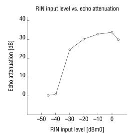
Measurement Conditions : RIN input = -10 dBm0 5 kHz band white noise Echo delay time  $T_D = 50$  ms ATT, GC, NLP = OFF Power supply voltage 5 V
