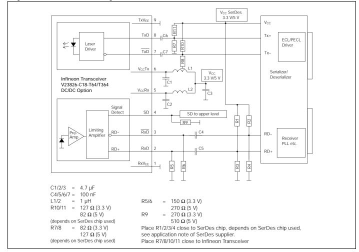
This Application Note assumes Fiber Optic Transceivers using 5 V power supply and SerDes Chips using 3.3 V power supply. It also assumes no self biasing at the receiver data inputs (RD+/RD-) of the SerDes chip (Refer to the manufacturer data sheet for other applications). 3.3 V-Transceivers can be directly connected to SerDes-Chips using standard PECL Termination network.
