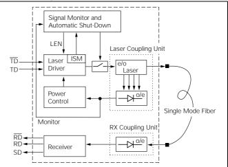
The transmitter converts electrical PECL compatible serial data (TD and TDnot) into optical serial data. It contains a laser driver circuit that drives the modulation and bias current of the laser diode. The currents are controlled by a power control circuit to guarantee constant output power of the laser over temperature and aging.
