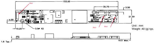
Note: Please use plastic screw in case of a non-insulating mounting base!
