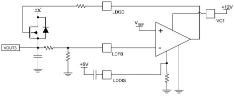
Figure 2 – LDO Controller Block Diagram
