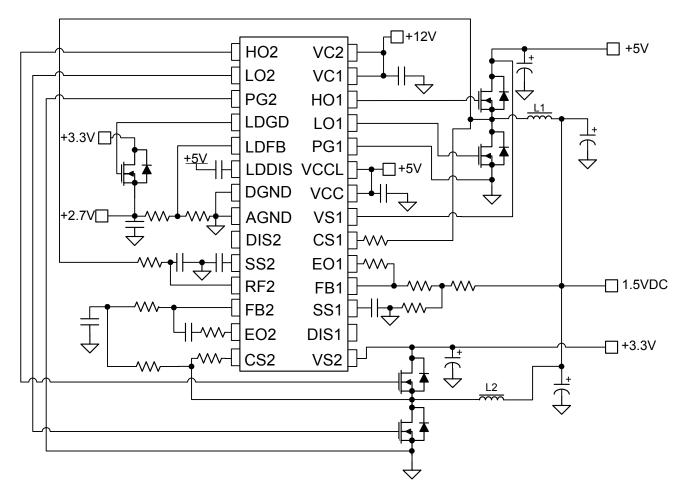
Figure 4 – Bi-Phase Operation With Phase 1 & 2 LoadSHARing From 5V & 3.3V
