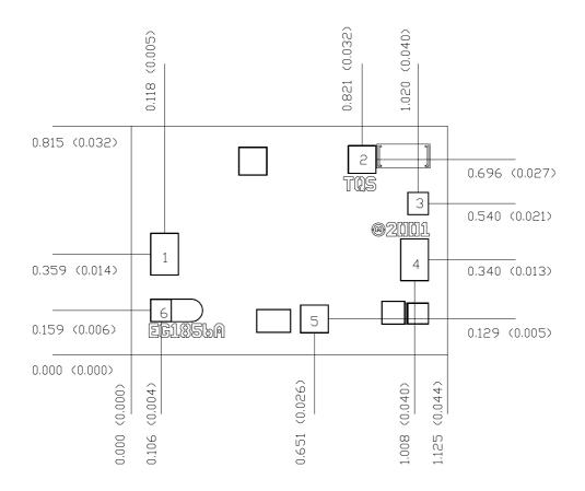
Units: millimeters (inches) Thickness: 0.1016 (0.004)
