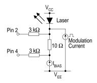
Figure 1. Laser Bias Monitor Circuitry
