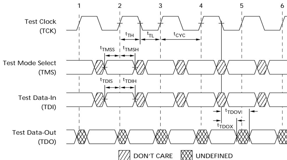
**TAP AC Switching Characteristics** Over the Operating Range<sup>[10, 11]</sup>
