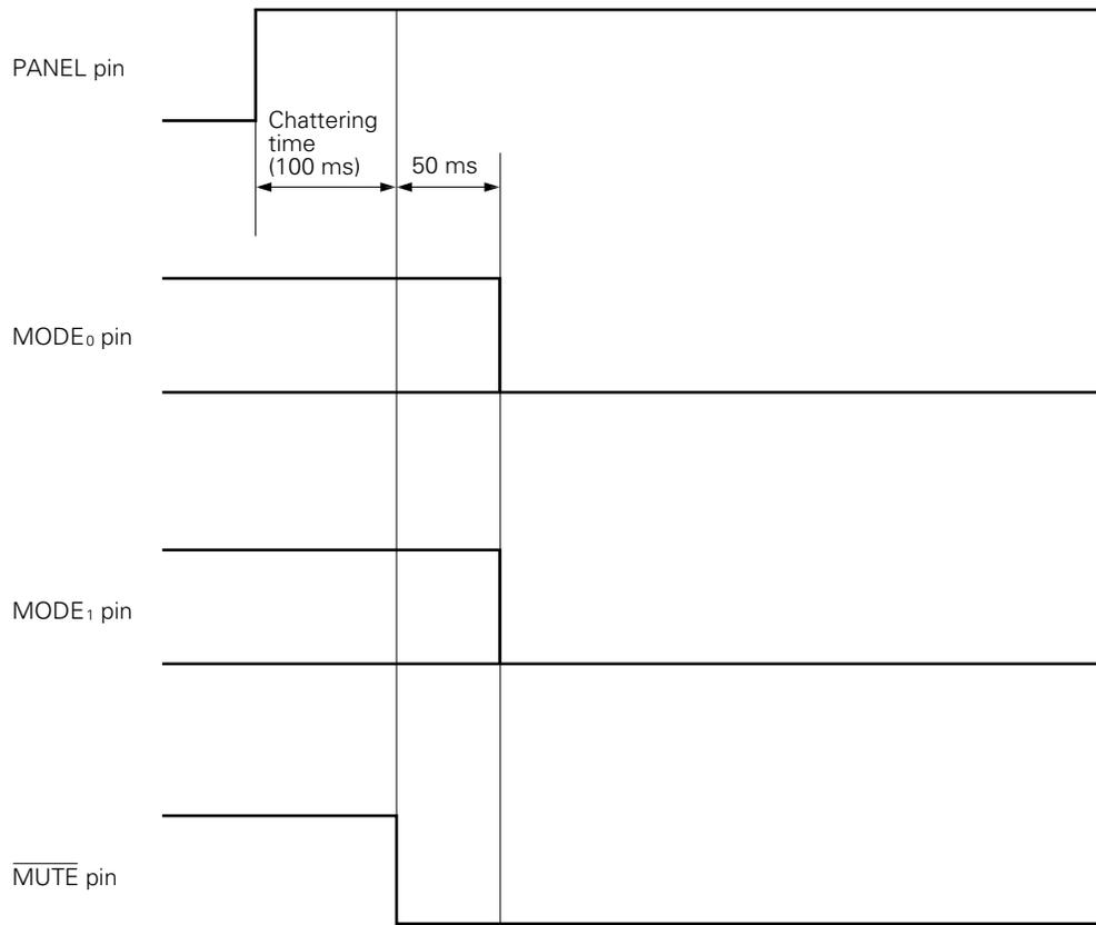
The mute output timing when the detachable panel is turned ON is the same as when the CE pin is turned ON.
