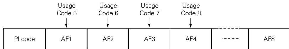
The storage positions corresponding to Usage Codes 5 to 8 are predetermined as shown in the above figure. AF1 takes the highest priority for AF selection. In this case, even if the AF list in a pool memory has been already registered, the pool memory is overwritten when Usage Codes 5 to 8 are input.
