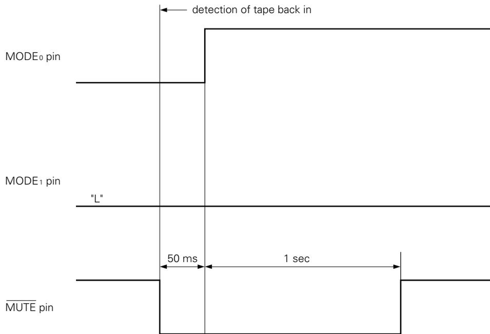
Sound mode selection mute output other than mode change within the same sound mode, such as a change between tuner mode and traffic information mode, is carried out as in the above timing (50 ms after the mute is output).
