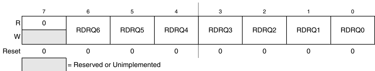
Figure 3-26. Port Q Reduced Drive Register (RDRQ)
