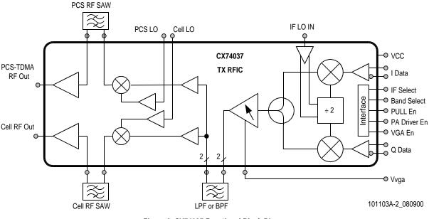
Figure 2. CX74037 Functional Block Diagram
