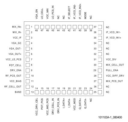
Figure 1. CX74037 48-Pin, 7x7 LGA Package Pin Configuration
