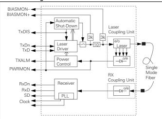
The receiver component converts the optical serial data into PECL compatible electrical data (RxD and RxDn). It provides also a recovered in-phase clock and clock not signal. The Signal Detect (SD, active high) shows whether an optical signal is present. If no optical input signal is present the receiver data outputs are switched to static low level (RD=low, RDnot=high).
