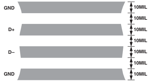
Figure 4. Arrangement of Signal Tracks
