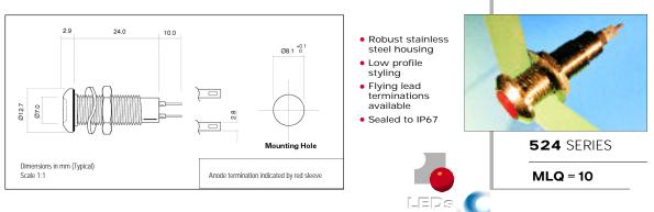
Ordering Information & Typical Technical Characteristics (Ta =  $25^{\circ}$ C) Mean Time Between Failure = 100,000 Hours. Luminous intensity figures refer to the unmodified discrete LED.
