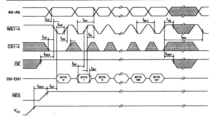
Note: A7 through A16 must specify the page address during each high to low transition of WE (or CS).
