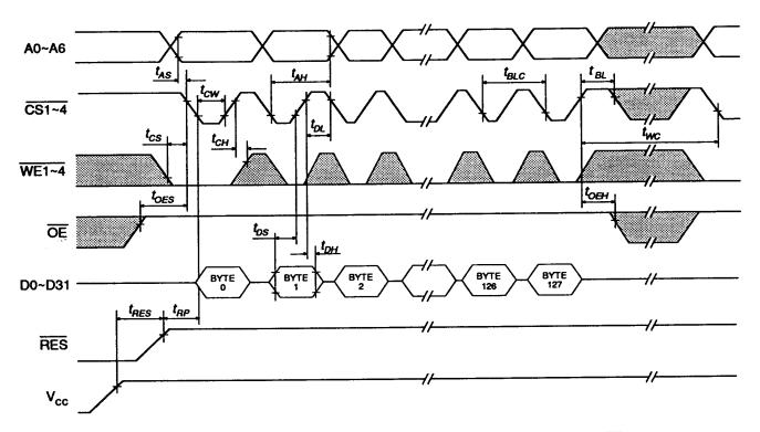
Note: A7 through A16 must specify the page address during each high to low transition of WE (or CS).
