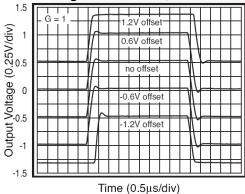
Figure 20. Pulse Response vs. Common Mode Voltage
