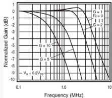
Figure 8. Non-Inverting Frequency Response
