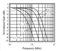
Figure 7. Inverting Frequency Response (+5V)
