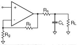
Figure 25. Typical Topology for Driving a Capacitive Load
