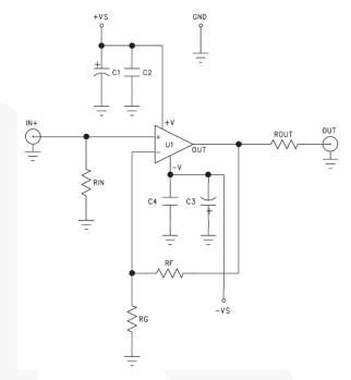
Figure 26. FAN4174 Evaluation Board Schematic (KEV002/KEB011)
