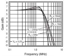
Figure 11. Frequency Response vs. RL
