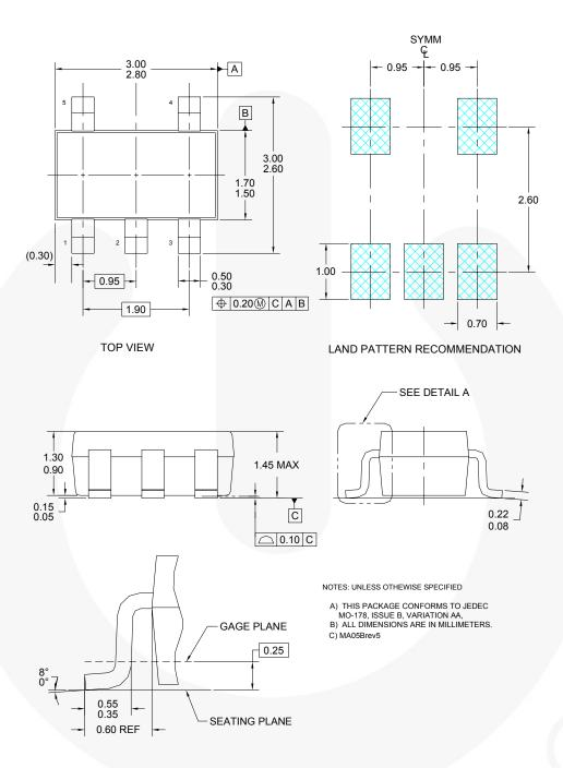
Figure 32. 5-Lead SOT-23 Package
