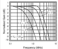
Figure 9. Inverting Frequency Response
