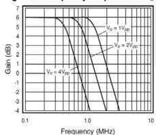
Figure 12. Large Signal Frequency Response (+5V)
