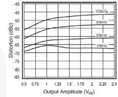
Figure 15. 2nd Harmonic Distortion vs. Vo
