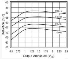
Figure 16. 3rd Harmonic Distortion vs. Vo
