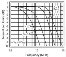
Figure 6. Non-Inverting Frequency Response (+5)
