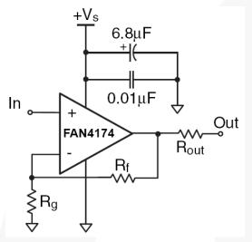
Figure 22. Typical Non-inverting Configuration
