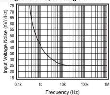
Figure 21. Input Voltage Noise
