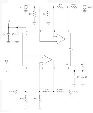
Figure 27. FAN4274 Evaluation Board Schematic (KEB010)
