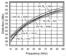
Figure 14. 2nd and 3rd Harmonic Distortion
