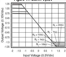
Figure 19. Output Swing vs. Load
