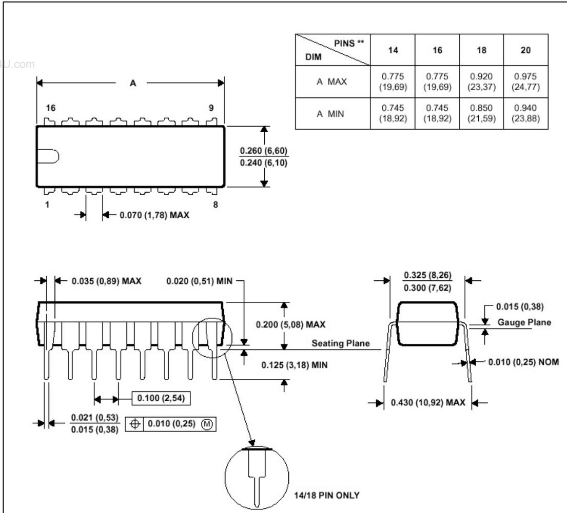
NOTE 1 : All linear dimensions are in inches ( millimeters ) .
