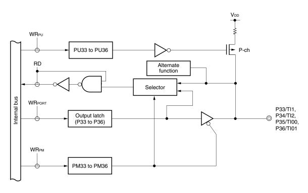
Figure 5-9. Block Diagram of P33 to P36
