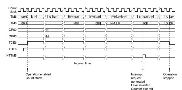
Figure 10-8. Cascade Connection Mode with 16-Bit Resolution
