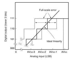
Figure 13-12. Integral Linearity Error
