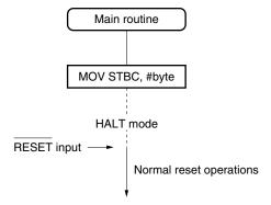
Figure 24-5. Operations After Releasing HALT Mode (2/4)
