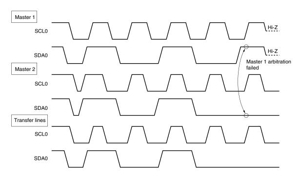
Figure 18-14. Example of Arbitration Timing
