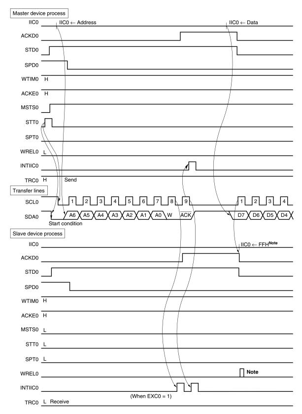
Figure 18-20. Master → Slave Communication Example (When Master and Slave Select 9 Clock Waits) (2/3)
