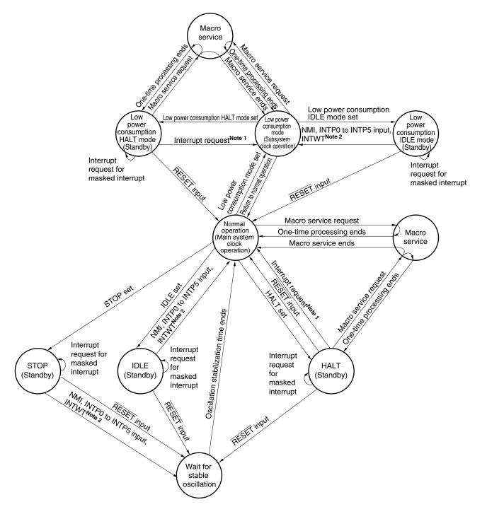
Figure 24-1. Standby Function State Transition
