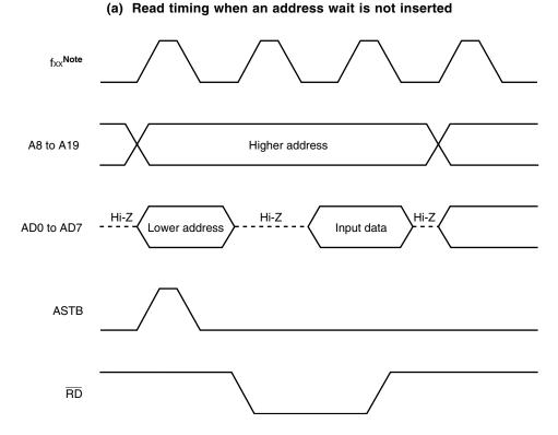
Figure 23-9. Read/Write Timing by Address Wait Function (2/3)
