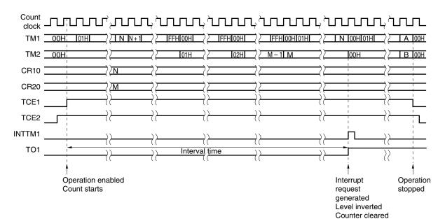
Figure 9-10. Cascade Connection Mode with 16-Bit Resolution
