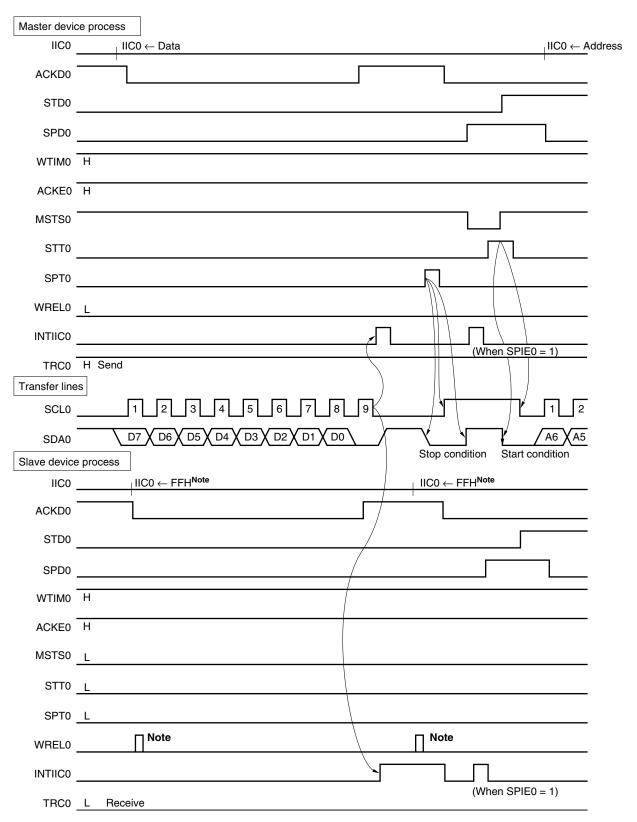
Figure 18-21. Slave → Master Communication Example (When Master and Slave Select 9 Clock Waits) (1/3)
