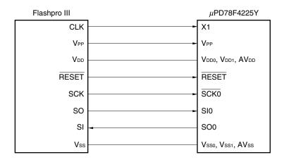
Figure 27-4. Connection of Flashpro III in 3-Wire Serial I/O Mode (When Using Handshake)
