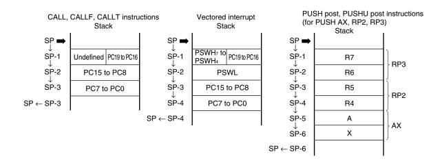
Figure 3-9. Data Restored from the Stack
