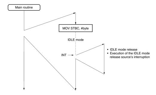
Figure 24-9. Operations After Releasing IDLE Mode (3/3)
