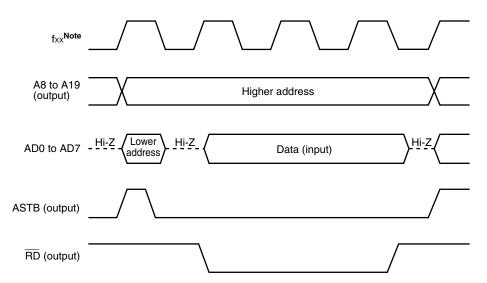
Figure 23-10. Read Timing by Access Wait Function (2/2)
