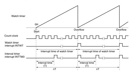
Figure 11-3. Operation Timing of Watch Timer/Interval Timer
