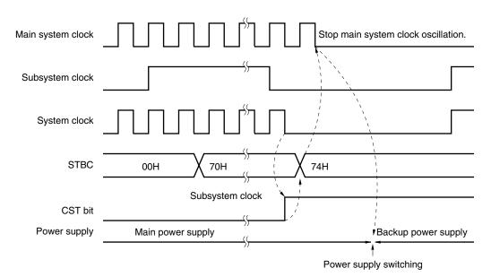
Figure 24-12. Setting Timing for Subsystem Clock Operation
