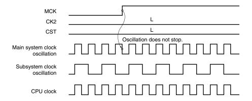
Figure 4-9. Main System Clock Stop Function (2/2)
