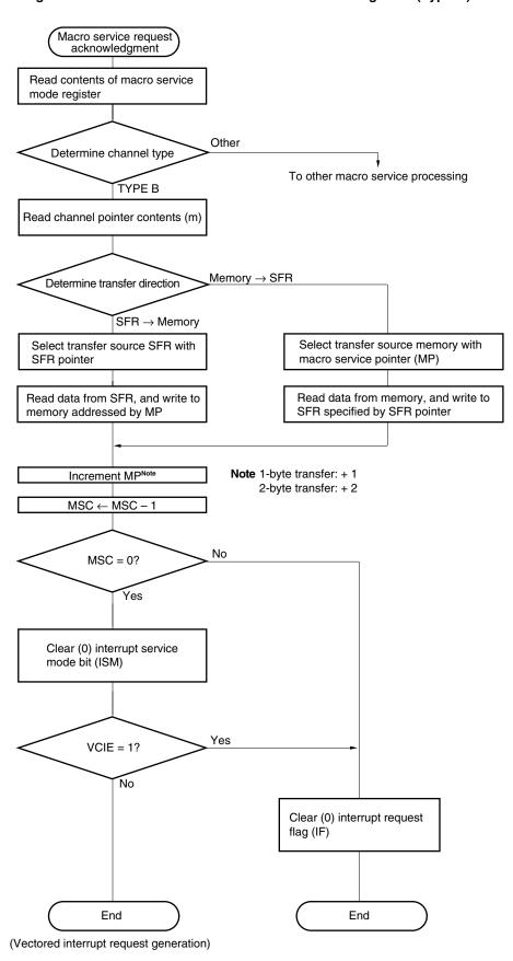
Figure 22-26. Macro Service Data Transfer Processing Flow (Type B)
