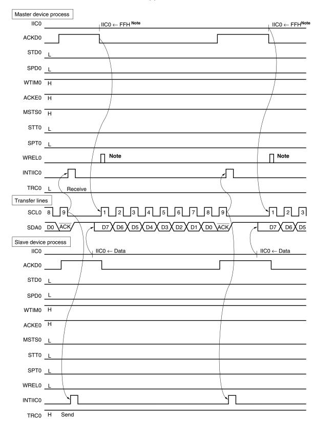
Figure 18-21. Slave → Master Communication Example (When Master and Slave Select 9 Clock Waits) (3/3)
