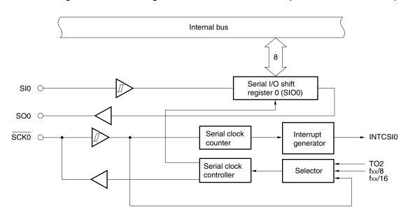
Figure 17-1. Block Diagram of Clocked Serial Interface (in 3-Wire Serial I/O Mode)
