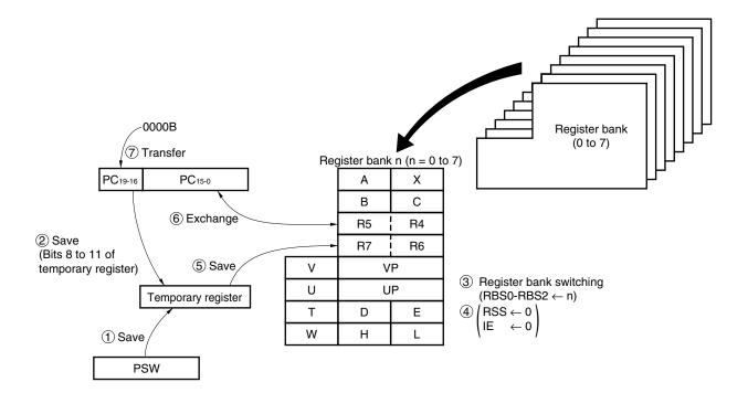
Figure 22-8. Context Switching Operation by Execution of a BRKCS Instruction
