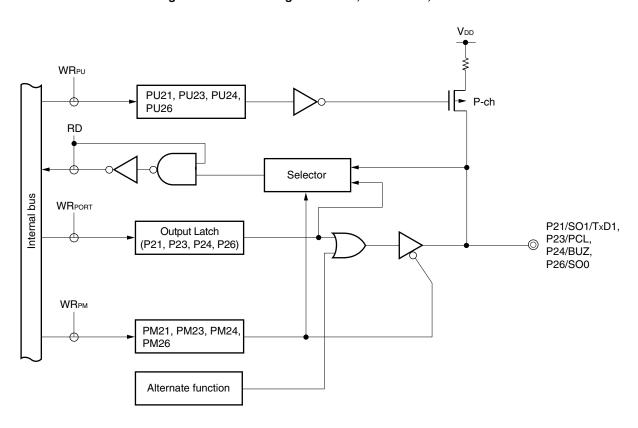
Figure 5-5. Block Diagram of P21, P23 to P24, and P26
