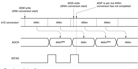
Figure 13-16. A/D Conversion End Interrupt Request Generation Timing
