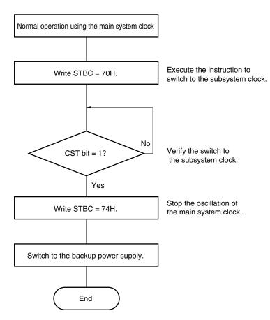
Figure 24-11. Flow for Setting Subsystem Clock Operation
