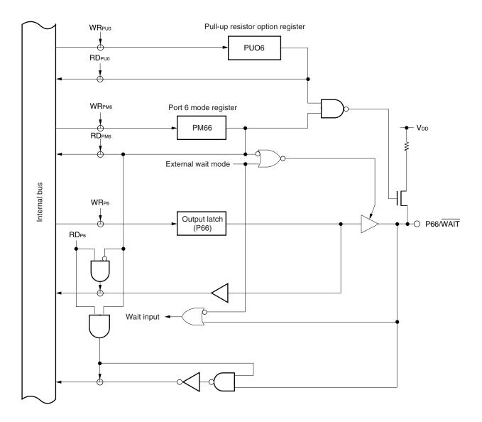
Figure 5-14. Block Diagram of P66
