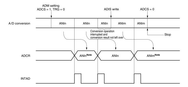
Figure 13-7. A/D Conversion Operation by Software Start
