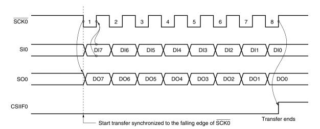
Figure 17-5. 3-Wire Serial I/O Mode Timing
