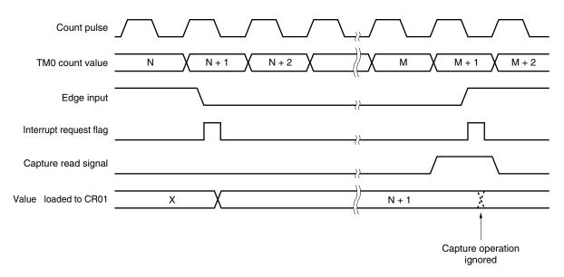
Figure 8-31. Data Hold Timing of Capture Register
