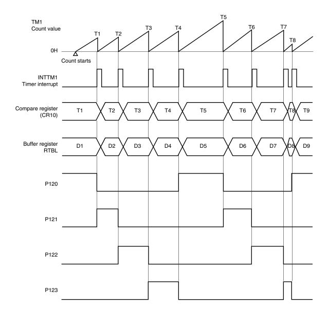
Figure 22-33. Data Transfer Control Timing
