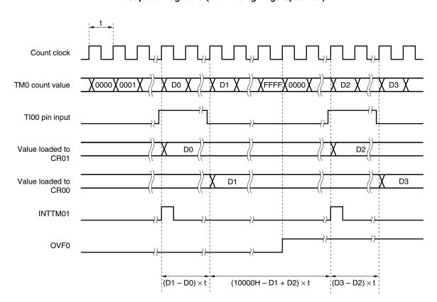
Figure 8-17. Timing of Pulse Width Measurement with Free-Running Counter and Two Capture Registers (with Rising Edge Specified)
