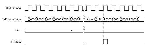
Figure 8-22. Timing of External Event Counter Operation (with Rising Edge Specified)
