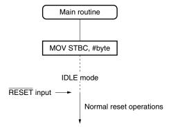
Figure 24-9. Operations After Releasing IDLE Mode (2/2)
