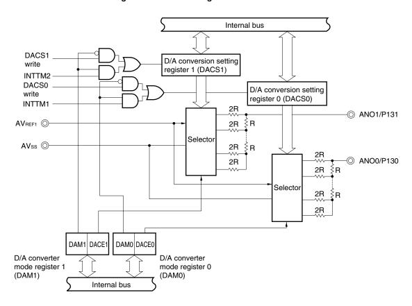
Figure 14-1. Block Diagram of D/A Converter
