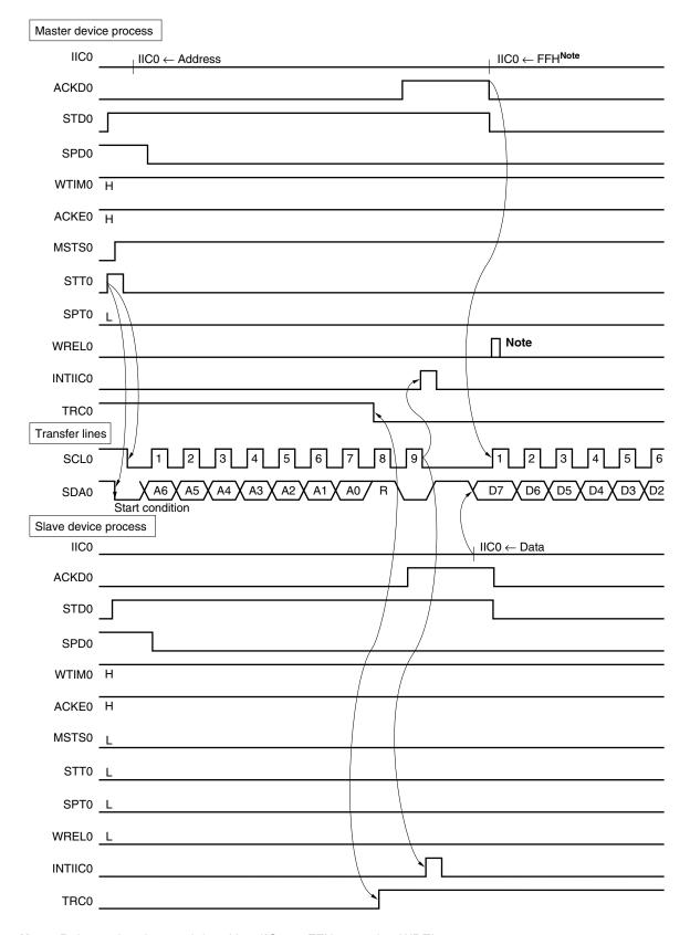
Figure 18-21. Slave → Master Communication Example (When Master and Slave Select 9 Clock Waits) (2/3)
