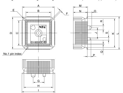
Figure B-2. Package Drawing of EV-9200GC-80 (Reference) (Unit: mm)
