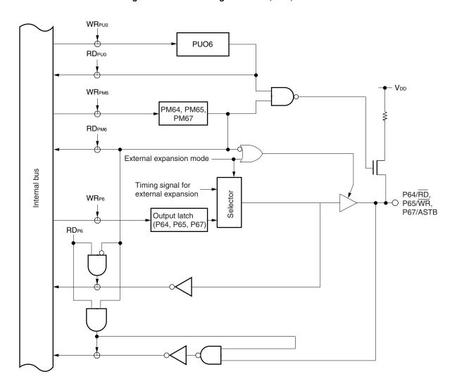
Figure 5-13. Block Diagram of P64, P65, and P67
