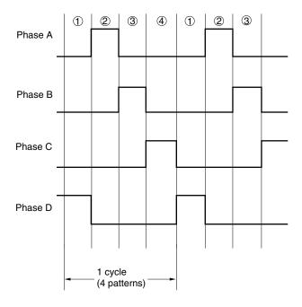
Figure 22-35. 1-2-Phase Excitation of 4-Phase Stepper Motor
