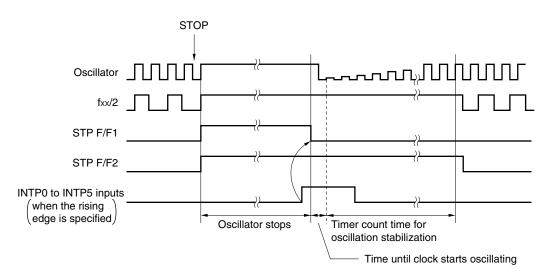
Figure 24-8. Example of Releasing STOP Mode by INTP0 to INTP5 Inputs
