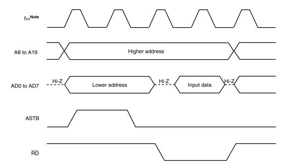
Figure 23-9. Read/Write Timing by Address Wait Function (3/3)
