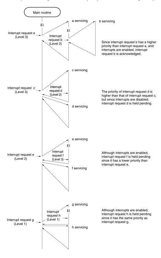
Figure 22-14. Examples of Servicing When Another Interrupt Request Is Generated During Interrupt Service (2/3)
