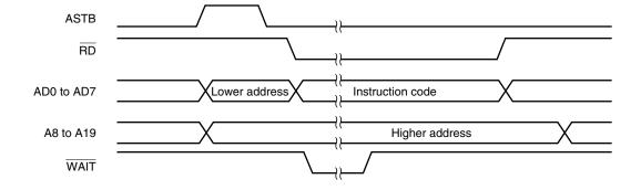
Figure 23-6. Read Timing for External Memory in External Memory Expansion Mode
