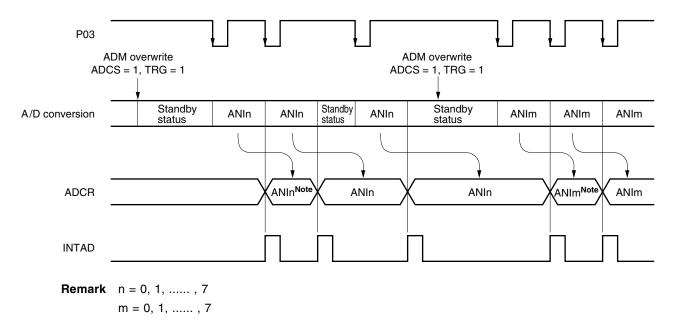
Figure 13-6. A/D Conversion Operation by Hardware Start (When Falling Edge Is Specified)
