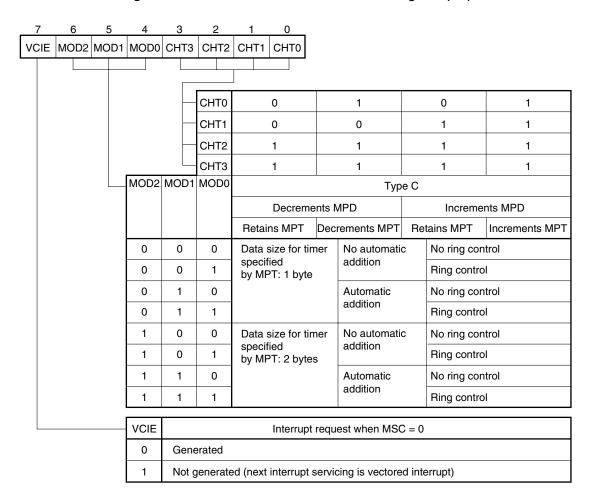
Figure 22-22. Format of Macro Service Mode Register (2/2)
