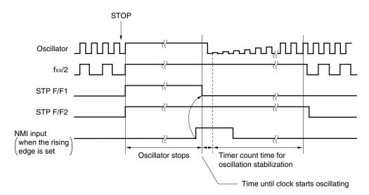
Figure 24-7. Releasing STOP Mode by NMI Input
