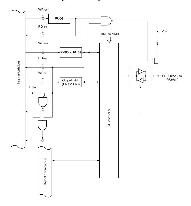
Figure 5-12. Block Diagram of P60 to P63
