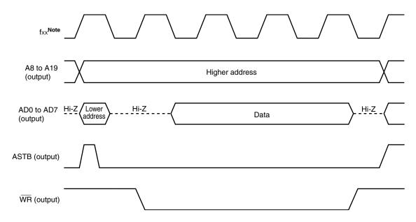
Figure 23-12. Timing by External Wait Signal
