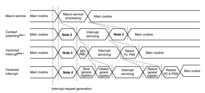
Figure 22-17. Differences Between Vectored Interrupt and Macro Service Processing
