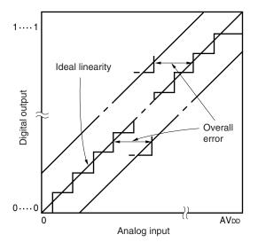
Figure 13-9. Quantization Error
