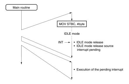
(4) IDLE mode during interrupt servicing routine whose priority is lower than release source interrupt
