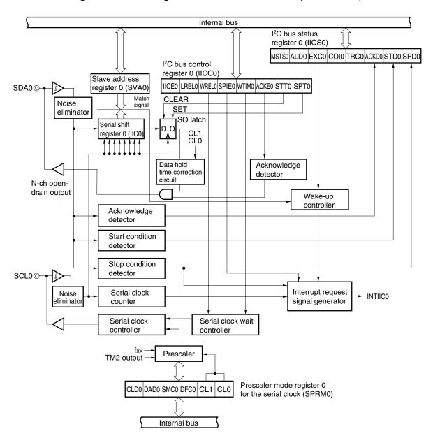
Figure 18-2. Block Diagram of Clocked Serial Interface (I<sup>2</sup>C Bus Mode)
