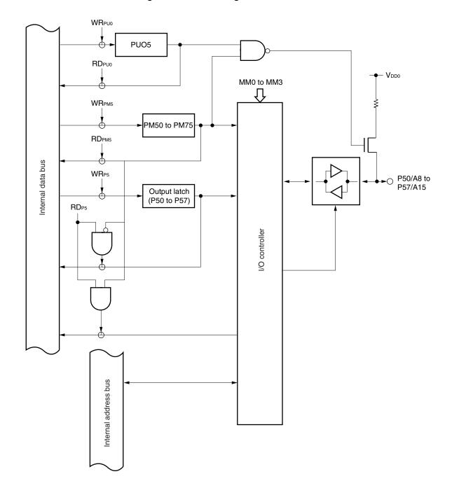
Figure 5-11. Block Diagram of P50 to P57
