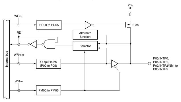
Figure 5-2. Block Diagram of P00 to P05
