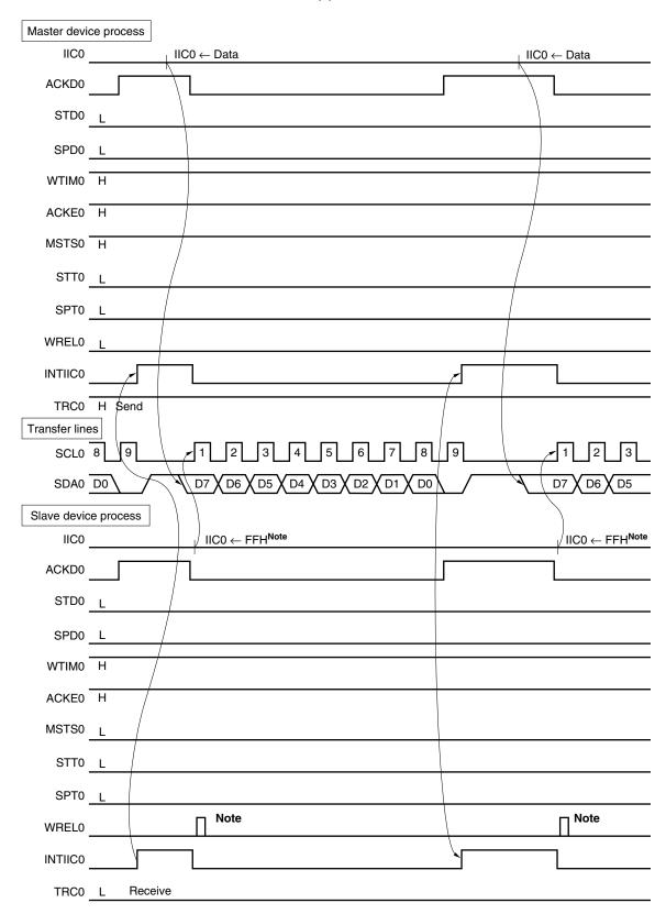
Figure 18-20. Master → Slave Communication Example (When Master and Slave Select 9 Clock Waits) (3/3)
