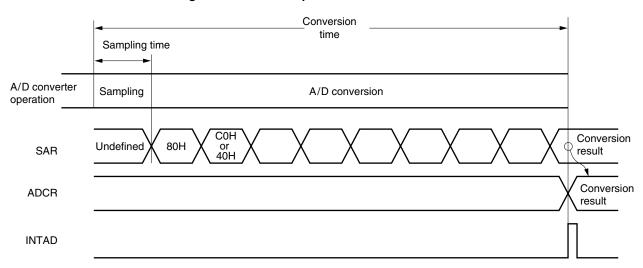
Figure 13-4. Basic Operations of A/D Converter
