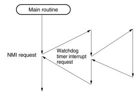
Figure 22-10. Non-Maskable Interrupt Request Acknowledgment Operations (2/2)
