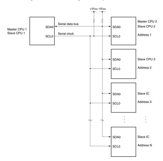
Figure 18-1. Serial Bus Configuration Example in I<sup>2</sup>C Bus Mode
