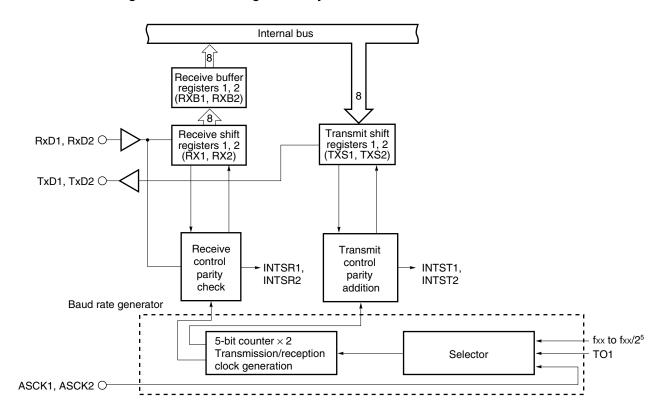
Figure 16-2. Block Diagram in Asynchronous Serial Interface Mode
