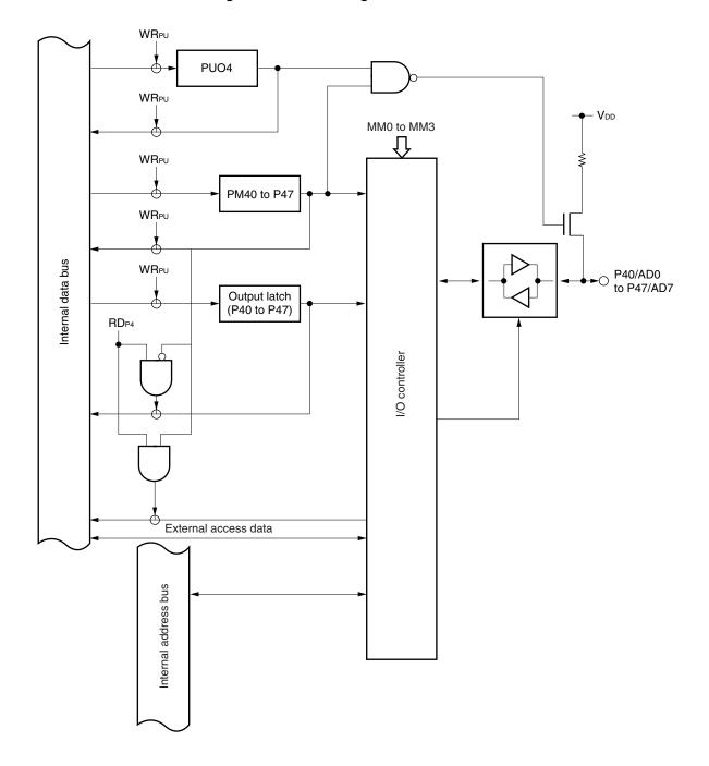
Figure 5-10. Block Diagram of P40 to P47
