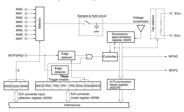
Figure 13-1. Block Diagram of A/D Converter
