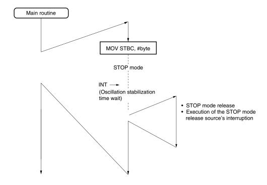
Figure 24-6. Operations After Releasing STOP Mode (3/3)
