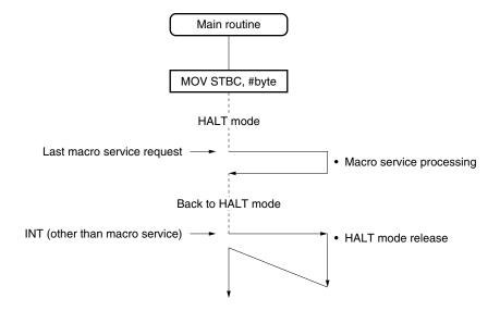
Figure 24-5. Operations After Releasing HALT Mode (4/4)
