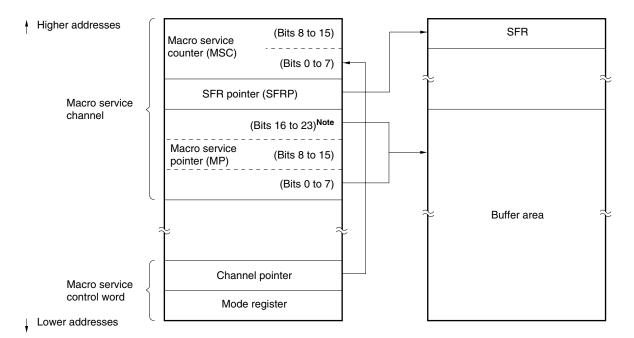
Figure 22-27. Type B Macro Service Channel
