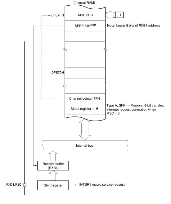
Figure 22-25. Asynchronous Serial Reception
