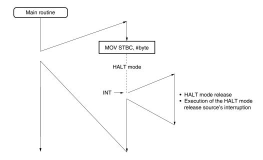
Figure 24-5. Operations After Releasing HALT Mode (3/4)
