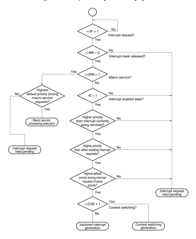
Figure 22-11. Interrupt Acknowledgment Processing Algorithm
