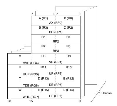
Figure 3-10. Format of General-Purpose Register
