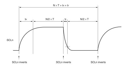
IIC clock frequency: fscL =  $1/(N \times T + tR + tF)$ T = 1/fxx, tR: SCLn rise time, tF: SCLn fall time **Example** When fxx = 12.5 MHz, N = 172, t<sub>R</sub> = 200 ns, t<sub>F</sub> = 50 ns IIC clock frequency:  $1/(172 \times 80 \text{ ns} + 200 \text{ ns} + 50 \text{ ns}) \cong 71.4 \text{ kHz}$
