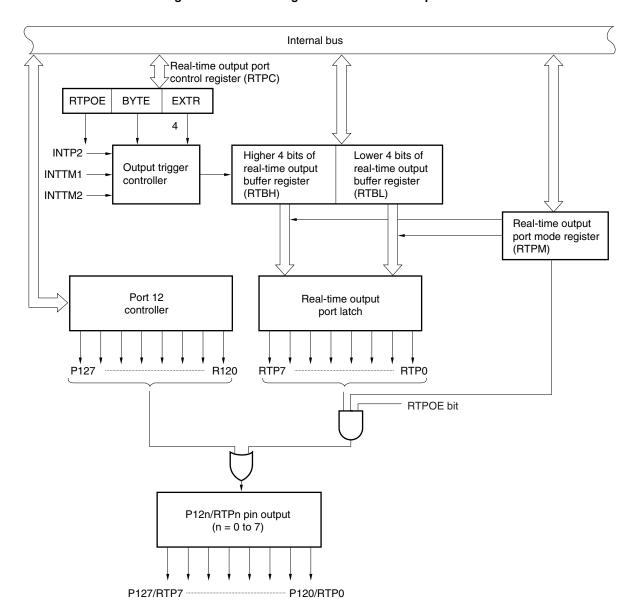
Figure 6-1. Block Diagram of Real-Time Output Port
