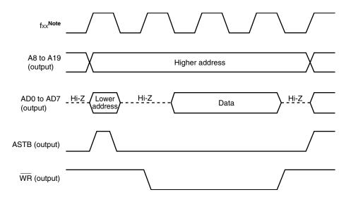
Figure 23-11. Write Timing by Access Wait Function (2/2)
