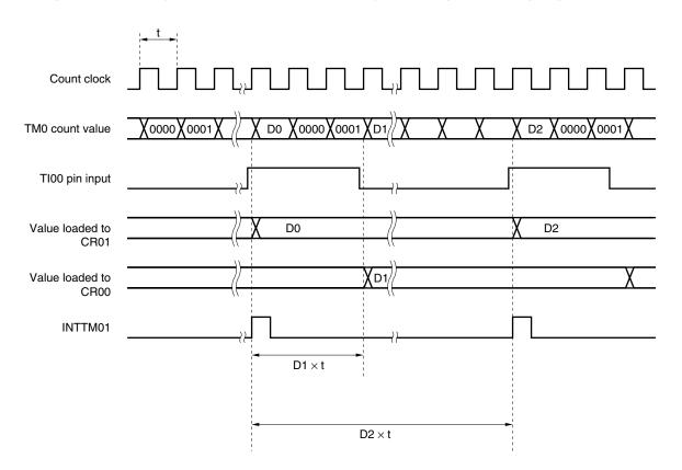
Figure 8-19. Timing of Pulse Width Measurement by Restarting (with Rising Edge Specified)
