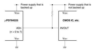
Figure 24-10. Example of Handling Address/Data Bus
