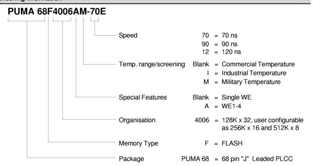
NOTE: The E variant is designated to parts with extended Erase/Write Cycle Endurance (100,000 Min.). If not specified when ordered only a Erase/Write Cycle Endurance of 10,000 Minimum can be guaranteed.
