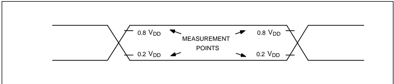
Figure 13-4. A.C. Timing Measurement Points (Except for  $X_{in}$ )
