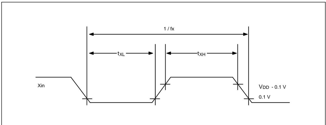
Figure 13-5. Clock Timing Measurement at  $X_{in}$
