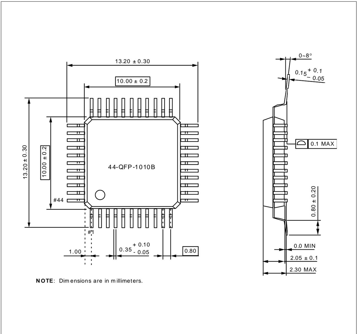
Figure 14-2. 44-QFP-1010B Package Dimensions
