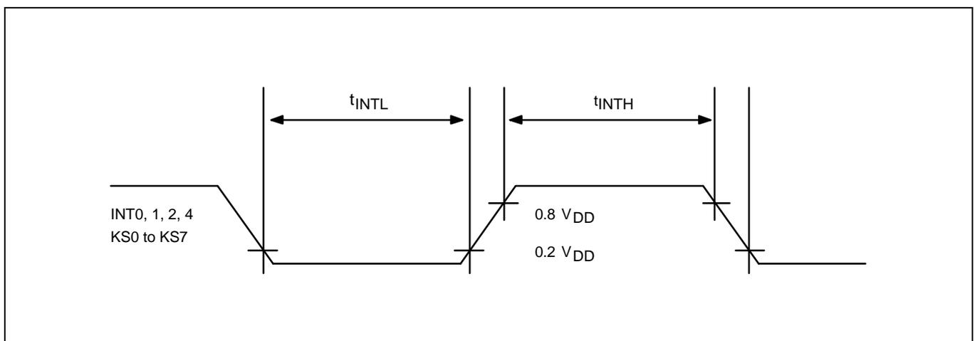
Figure 13-8. Input Timing for External Interrupts and Quasi-Interrupts
