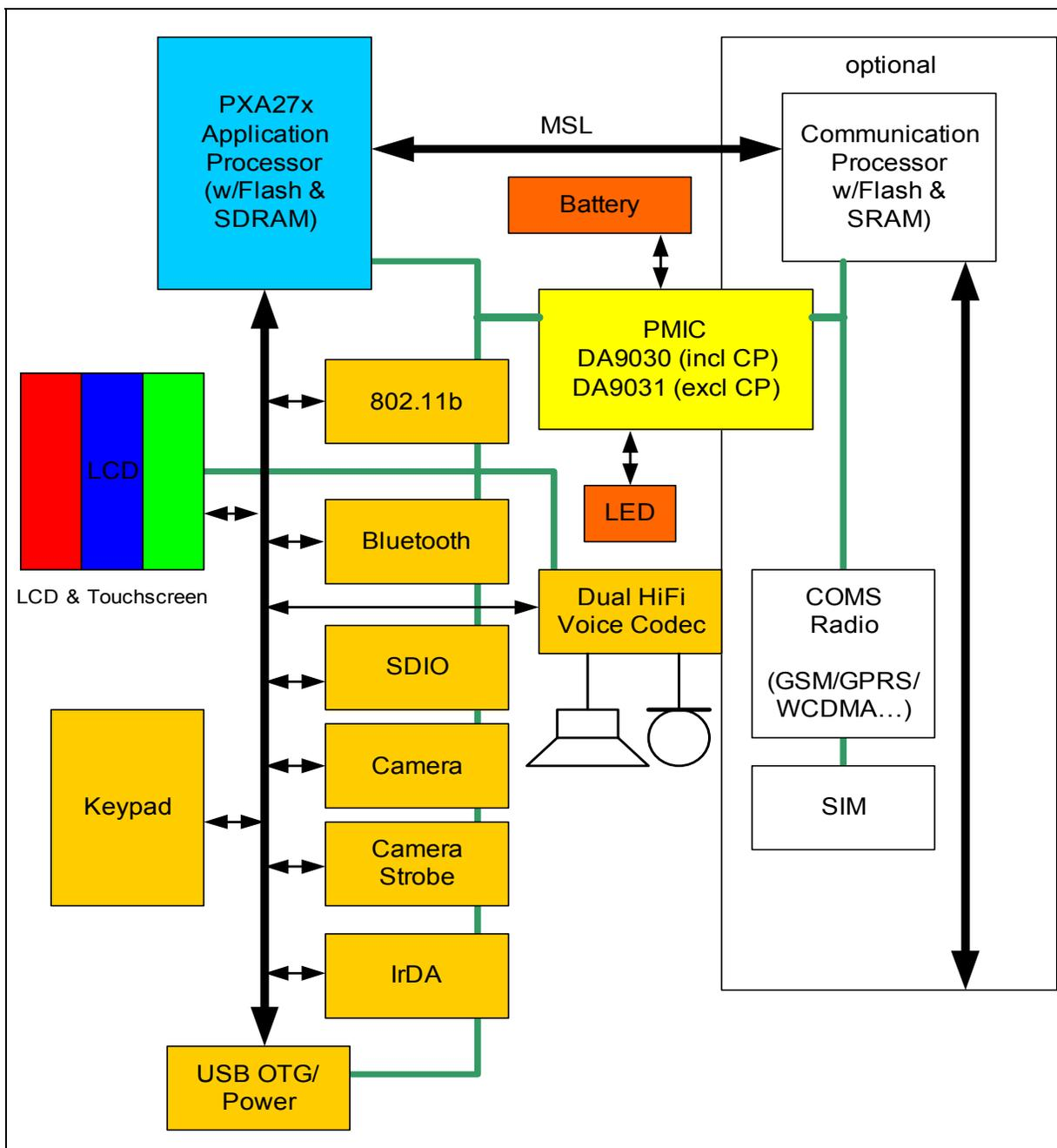
The system-application block diagram outlines a mobile handset using the PXA27x processor. The Dialog Semiconductor DA9030 PMIC handles all required power supplies for the PXA27x processor within such a system and also controls an (optional) communications processor (referred to in the remainder of this document as CProc) as well as the application processor, independently.
