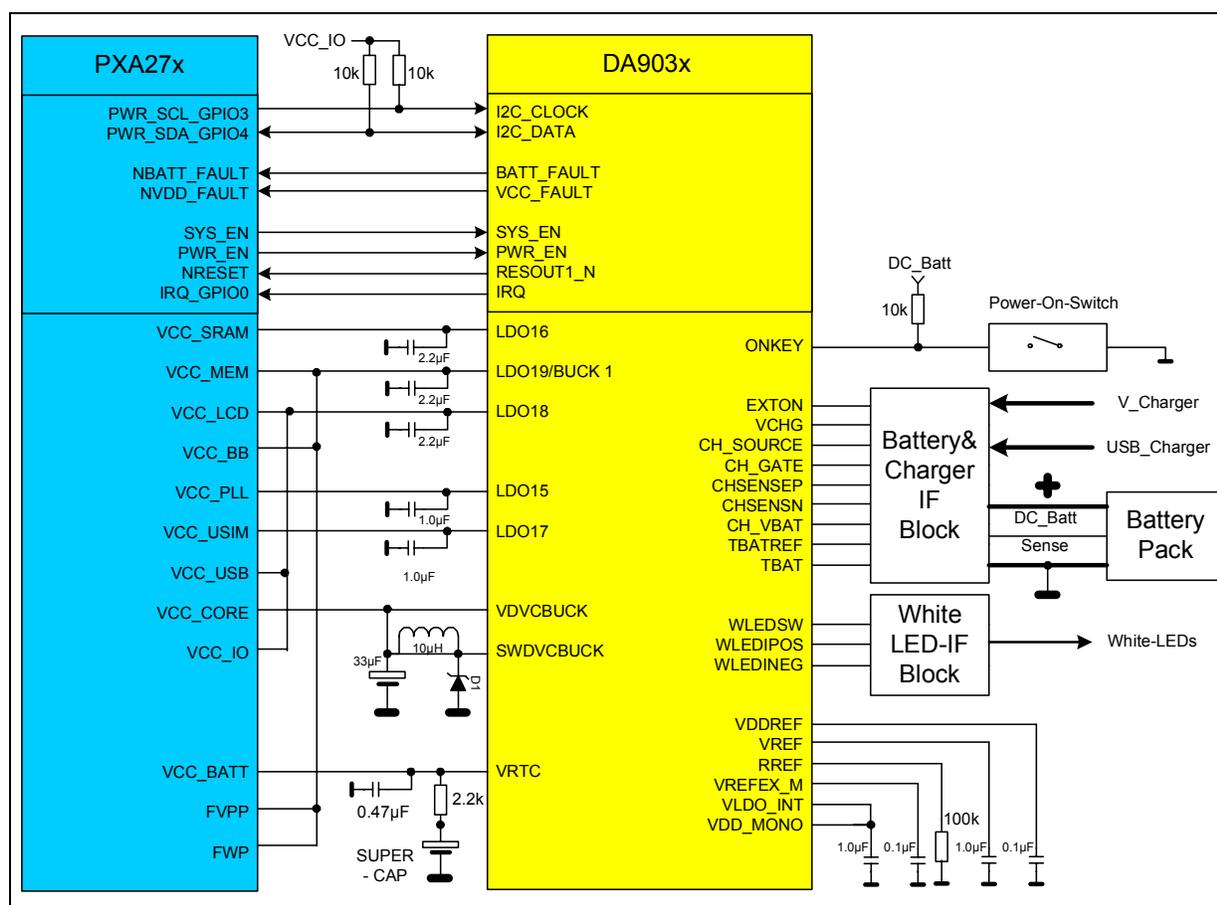
The schematic diagram in Figure 1 shows how the PXA27x processor and the DA903x can be interconnected to build an efficient power-supply system with few additional components. This configuration is set up for dynamic-voltage management as well as for supporting sleep mode. The white LED backlight circuit is optional.
