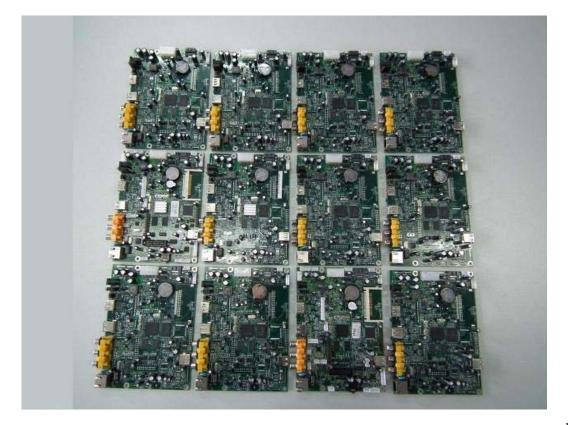
28. STB in mass production (PV8900-FULL board is build-in and connect to SSD HDD through SATA interface):
