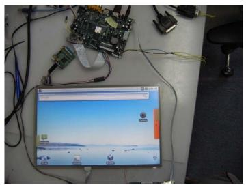
17. 17" LCD Panel M170E5-L09 Rev.C3 (1280\*1024, 4:3) display (Windows CE OS) through on board 24bit color dual channels LVDS port + CCFL inverter:
