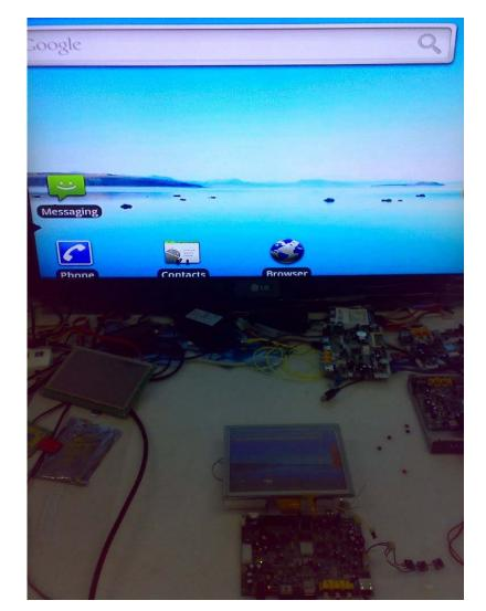
21. Dual display mode: Display the 8" LCD Panel's UI to 42" LCD TV through HDMI (Android):
