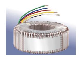
The SRT series is our latest development in toroidal transformers. They differ in design from traditional toroidal transformers as the advanced core construction produces characteristics similar to that of R-cored transformers. The improved rounded section of the core leads to a substantial reduction in flux leakage, therefore vigorously improving the units performance.
