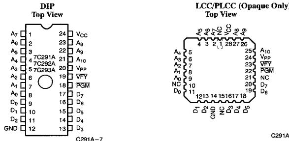
Figure 1. Programming Pinouts
