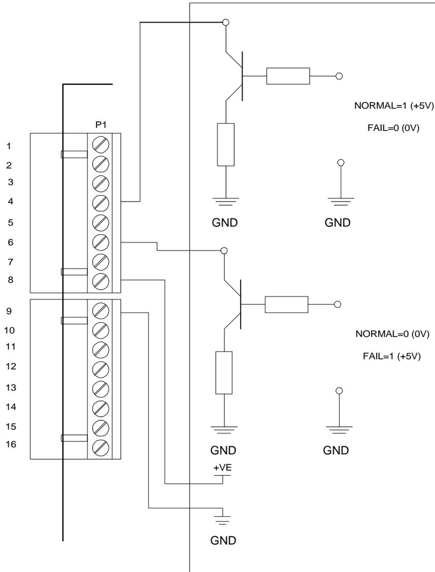
**Fig.6.5 Remote level inputs with INPUT1 non-inverting and INPUT2 inverting**
