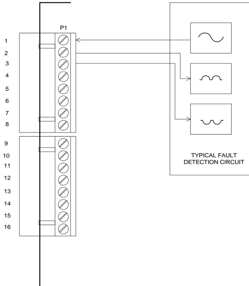
Fig.6.2 Using RL1 with fault detection circuitry
