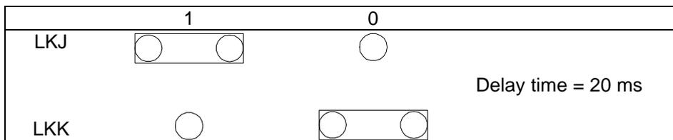
The watchdog channel has an additional link, LKL. This link allows the watchdog facility to be installed automatically from start up after a preset delay to allow the system to access its software. This is offered for applications where processor integrity is imperative. Alternatively, the watchdog facility may be installed manually i.e. through the WD-1 TSR software. The link arrangement is as shown below.
