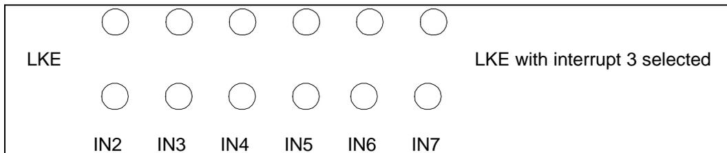
**N.B.** IN3 is selected at the Blue Chip Technology factory and the WD-1 TSR software defaults to this setting.
