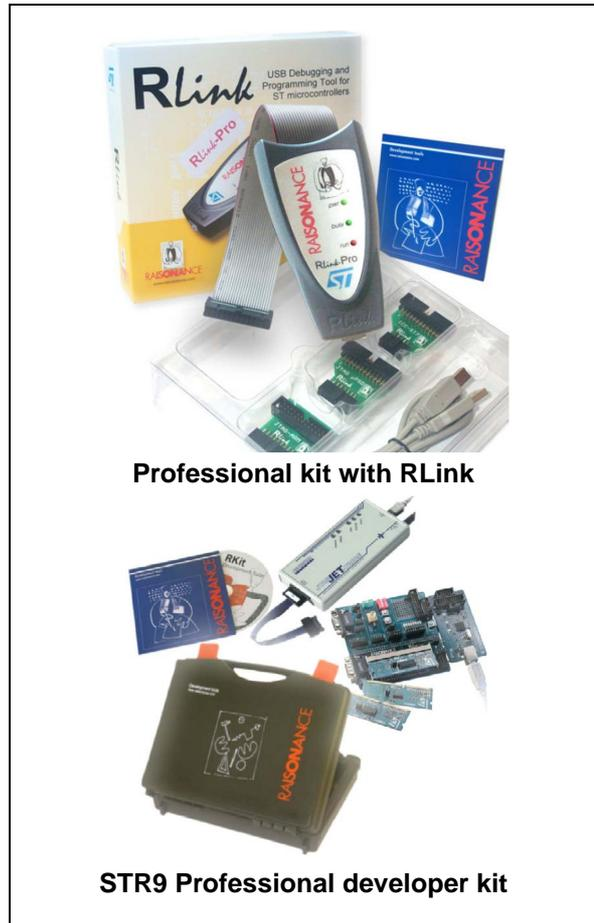
The tools contain everything required to develop STM32 and STR7/9 applications including in-circuit debugger/programmer, Raisonance Integrated Development Environment (RIDE) and GNU C/C++ compiler.
