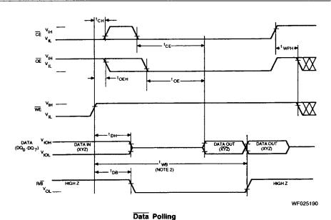
Notes: 1. This is shown for single byte write. In page write,  $R/\overline{B}$  goes LOW on first LOW-to-HIGH transition of  $\overline{WE}$ .
