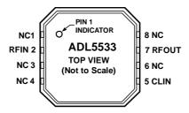
Figure 2. Pin Configuration
