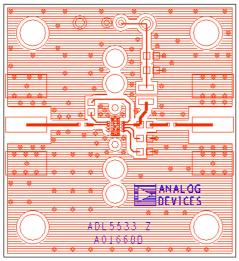
Figure 7. Evaluation Board Layout (Top)
