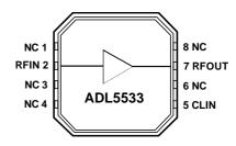
Figure 1. Block Diagram
