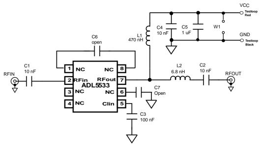
Figure 6. Evaluation Board Schematic
