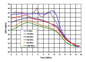
Figure 4 ADL5534 OIP3 vs Pout and Frequency
