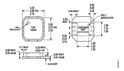
Figure 9. 8-Lead Lead Frame Chip Scale Package [LFCSP\_VD] 3mm × 3 mm Body, Very Thin, Dual Lead CP-8-2 Dimensions shown in millimeters
