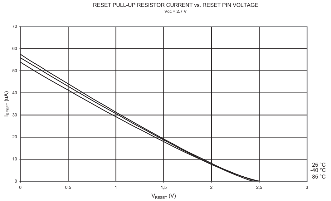
Figure 23-14. Reset Pull-up Resistor Current vs. Reset Pin Voltage ( V_{CC} = 2.7V )
