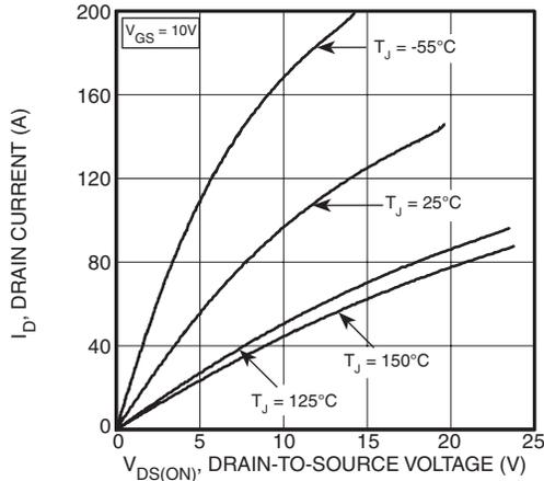
Figure 1, Output Characteristics
