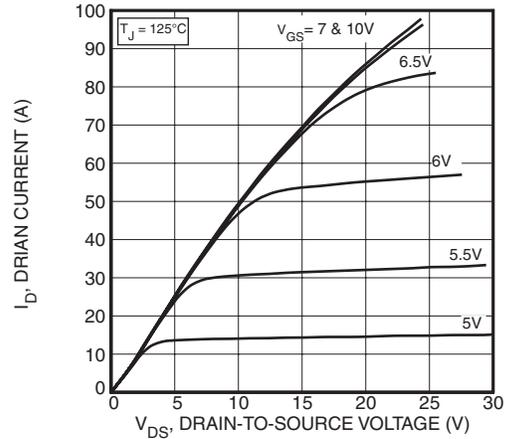
Figure 2, Output Characteristics
