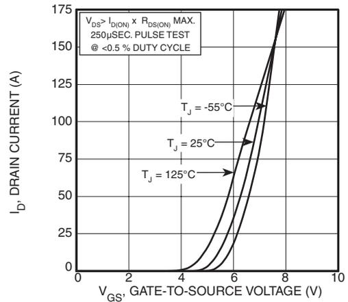
Figure 4, Transfer Characteristics
