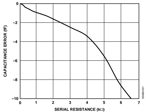
Figure 15. Capacitance Input Error vs. Serial Resistance, C_{IN(+)} \text{ to } EXC = 21 \text{ pF} , C_{IN(-)} \text{ to } EXC = 23 \text{ pF} , V_{DD} = 5 \text{ V} , the Same Configuration as in Figure 34.
