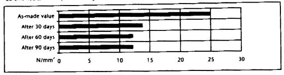
Fatigue test on simple lap joints (DIN 53285)
