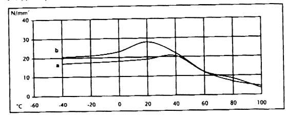
Roller peel test (ISO 4578) Cured 16 hours/40°C 5 N/mm
