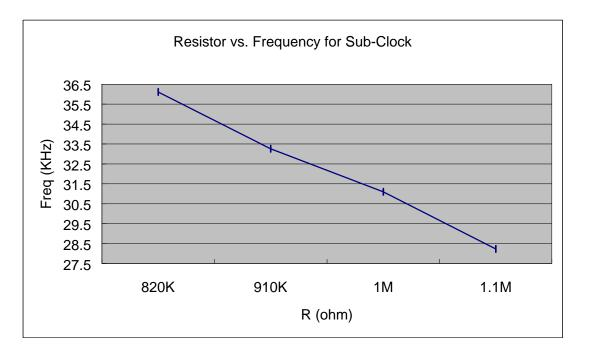
• Resistance vs. Frequency for W566B210/B260/B300/B340 at VDD = 4.5V, sub-clock in RC Type
