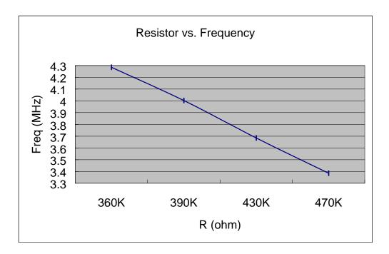
• Resistance vs. Frequency for W566B210/B260/B300/B340 at VDD = 4.5V, main-clock in Ring Type
