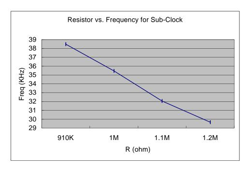
• Resistance vs. Frequency for W566B060/B080 at VDD = 4.5V, sub-clock in RC Type
