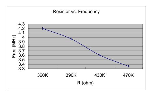
• Resistance vs. Frequency for W566B025/B030/B040 at VDD = 4.5V, main-clock in Ring Type
