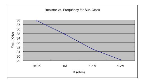
• Resistance vs. Frequency for W566B025/B030/B040 at VDD = 4.5V, sub-clock in RC Type
