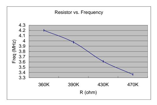
• Resistance vs. Frequency for W566B060/B080 at VDD = 4.5V, main-clock in Ring Type
