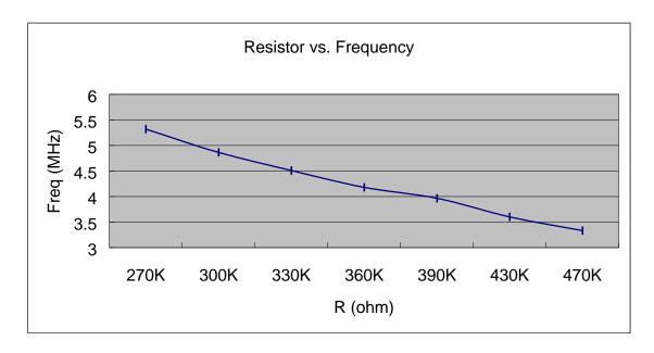
• Resistance vs. Frequency for W566B100/B120/B150/B170 at VDD = 3.0V, sub-clock in RC Type
