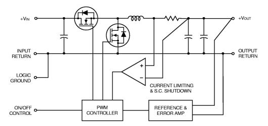
Signals applied to the On/Off Control are referenced to Logic Ground which is internally connected to Input/Output Return. The Logic Ground pin is not designed to carry heavy current. Do not install units with the Return pins open or connected via high-impedance runs.
