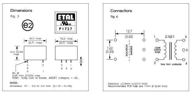
Dimensions shown are in millimetres (inches). Geometric centres of outline and pin grid coincide within a tolerance circle of 0.6mm
