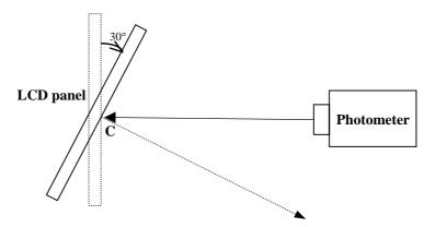
The LCD panel is then rotated to azimuthal angle to -30°; and  $L_{0~G.~L.,~-30}$ ° and  $L_{255~G.L.,~-30}$ ° are obtained by using the same procedure. The Luminance Contrast (Cm) is calculated:
