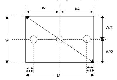
Luminance is measured at the center measurement position "C" on the LCD panel. The optical axis of the luminance meter shall be aligned with the normal of the panel surface. The measuring distance between the photometer and the surface of the panel is defined as:
