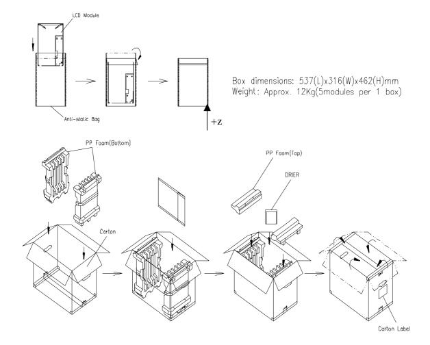
Figure. 8-1 Packing method
