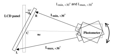
The LCD panel is then rotated to another azimuthal angle to -30°; and  $L_{min. -30}$ ° and  $L_{max. -30}$ ° are obtained by using the same procedure.
