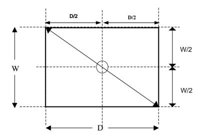
Luminance contrast is measured at the center point of the LCD panel "C" along with the normal of the display with the same distance described in Note 13. The display is then rotated around the vertical axis by changing its azimuthal axis to +30°; and this gives:
