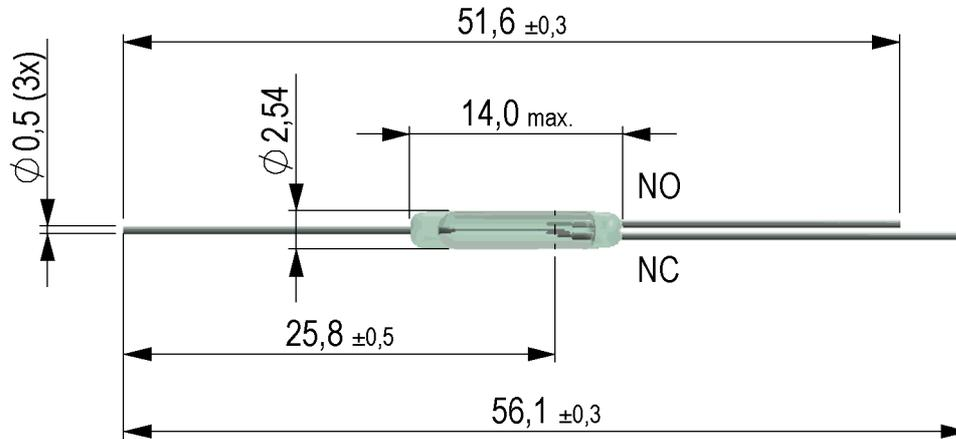
tolerances according to DIN ISO 2768 m
