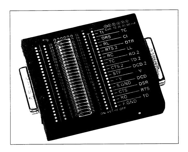
Comtests are constructed by field service engineers and famous for their convenience in use and reliability. They are the result of many years' experience in designing and incorporating customers' requests. The logical "in-line" design (switches, breakout, monitor, description on same height) make our BOBs the most compact and easy to read on the market.
