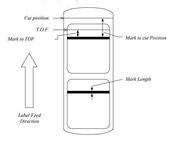
$\underline{\text{NOTE}}$ : Make sure that Hole/Black mark fully covers the opto sensor window, according to the paper path chosen (front or bottom).
