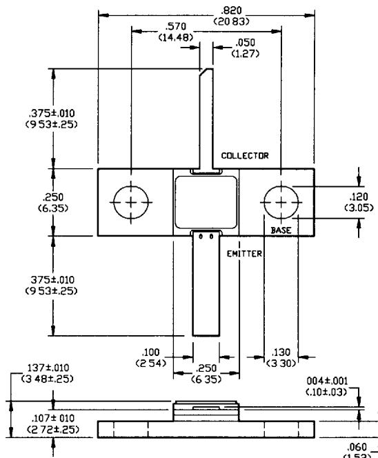
UNLESS OTHERWISE NOTED, TOLERANCES ARE INCHES ±005" (MILLIMETERS ±13MM)
