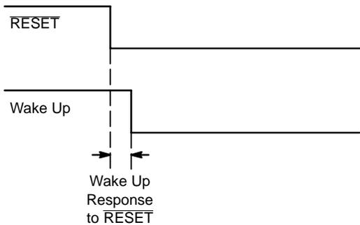
Figure 6. Wake Up Response to RESET (Low Voltage)
