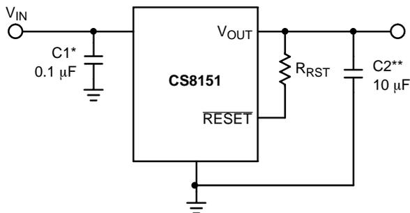
\*C1 required if regulator is located far from the power supply filter.
