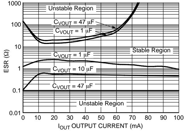
**Figure 11. CS8151 Output Stability with Output Capacitor Change**
