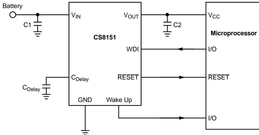
**Figure 10. Application Diagram**
