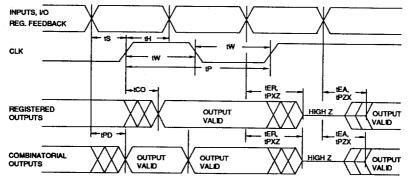
Note: 1. Timing measurement reference is 1.5 V. Input AC driving levels are 0.0 V and 3.0 V, unless otherwise specified.
