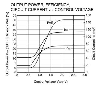
Condition: f = 2,450 MHz, Vcc1 = Vcc2 = Vbias = 3.3 V, Venable = 2.9 V, Vcont = 2.5 V, External input and output matching
