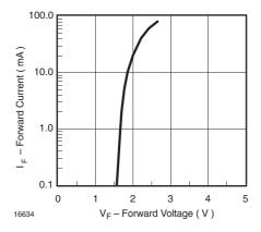
Figure 5. Forward Current vs. Forward Voltage
