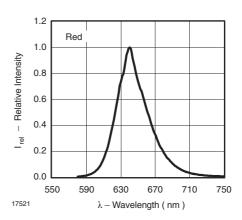
Figure 8. Relative Intensity vs. Wavelength
