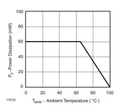
Figure 1. Power Dissipation vs. Ambient Temperature
