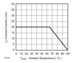
Figure 2. Forward Current vs. Ambient Temperature
