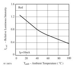
Figure 6. Rel. Luminous Intensity vs. Ambient Temperature
