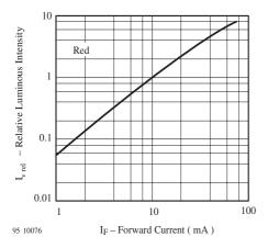
Figure 7. Relative Luminous Intensity vs. Forward Current
